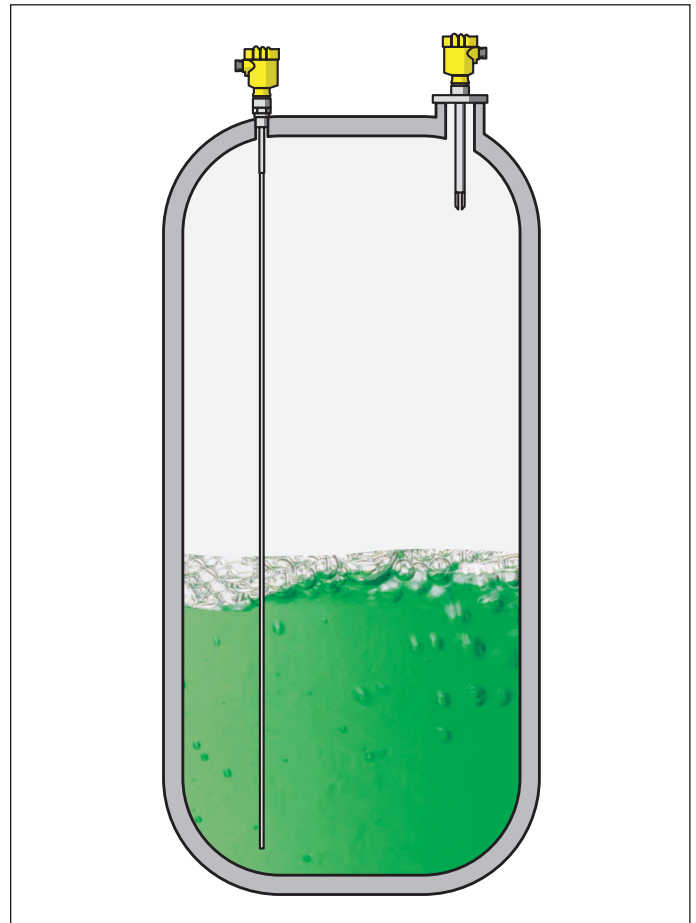
Fig. 2: Level detection in vessels with solvents
